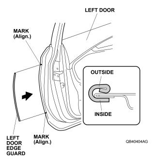
8. Using a rubber mallet, tap the left door edge guard into position with a series of light taps, then work up and down. Make sure the position of the left door edge guard is correct. Once in place, do not attempt to remove, reposition, or reinstall the left door edge guard.
